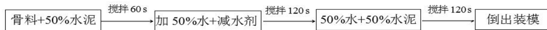
图 5 植生型再生砖瓦混凝土的搅拌工序 Fig.5 The mixing process of plant-growing concrete with recycled rubble
