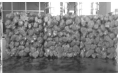
图 7 制备成功的多孔混凝土侧面图 Fig.7 The lateral view of prepared porous concrete
