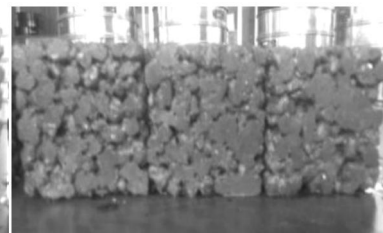
图 8 制备成功的多孔混凝土的底部图 Fig.8 The bottom diagram of prepared porous concrete
