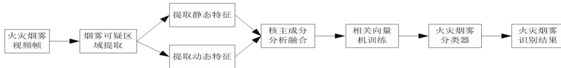
图 1 MF-RVM 的取火灾烟雾识别框图 Fig.1 The process of recognizing fire smog with MF-RVM
